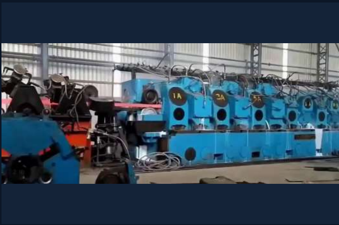
Copper CCR | Rolling line
