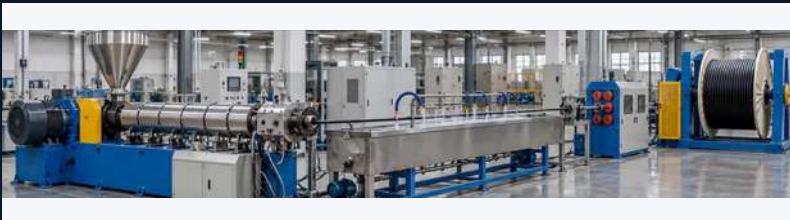
Cable Extrusion Line
