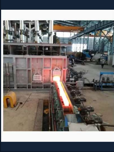
Billet Reheating Furnace Ejector
